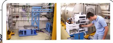
The insertion of the set-up within the X-ray beam path is facilitated by the large amount of space available around the motorized table for sample environments.
