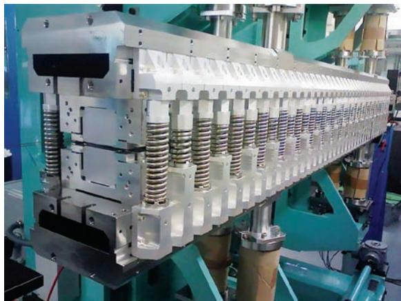
Figure 1. Wiggler multi-pôles WS50.
