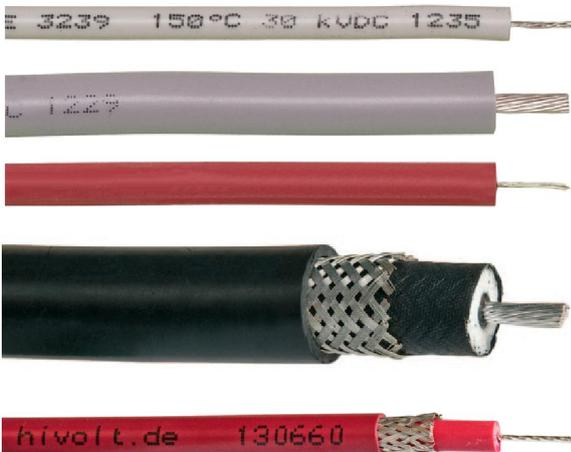
We offer unshielded and shielded coaxial cables for voltages up to 150 kV. The standardized offer contains Silicone and PE dielectrics, but miscellaneous dielectrics with good AC ratings are available too.
