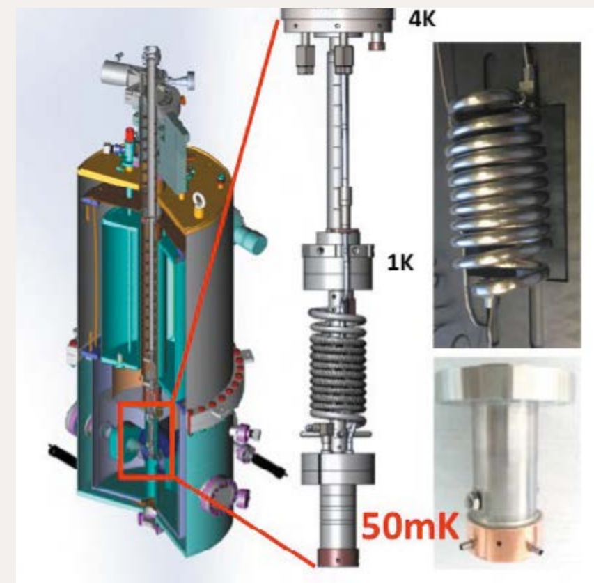
Figure 1 - 3D projection of DEIMOS cryomagnet, details of the low temperature stages of the device; right: pictures of the components before assembly (courtesy of Cryoconcept)
