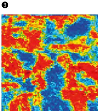
**Figure 3:** Coexistence of metallic (red) and insulating (blue) phases observed by X-ray spectromicroscopy. The image covers an area of  $50 \times 50 \mu\text{m}^2$ .
