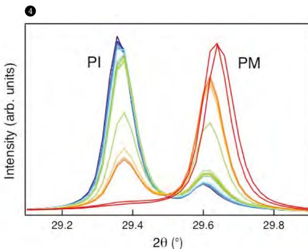
**Figure 4:** The metal-insulator transition observed by X-ray diffraction. Starting from the insulating phase (PI, blue), only the metallic phase (PM, red) remains at high-pressure.
