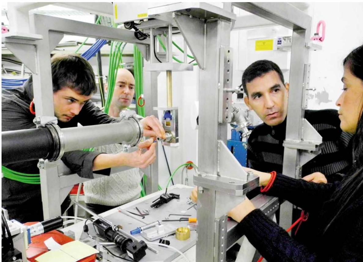
Installation of the electrochemical cell on ODE beamline.
