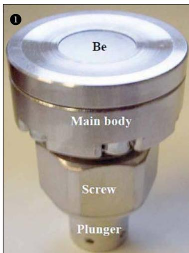
Figure 2: Electrochemical cell designed for operando experiments
