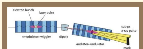
Figure 1: Sketch showing the principle of bunch slicing to generate femtosecond pulses of synchrotron radiation. From S. Khan, EPAC 2002.
