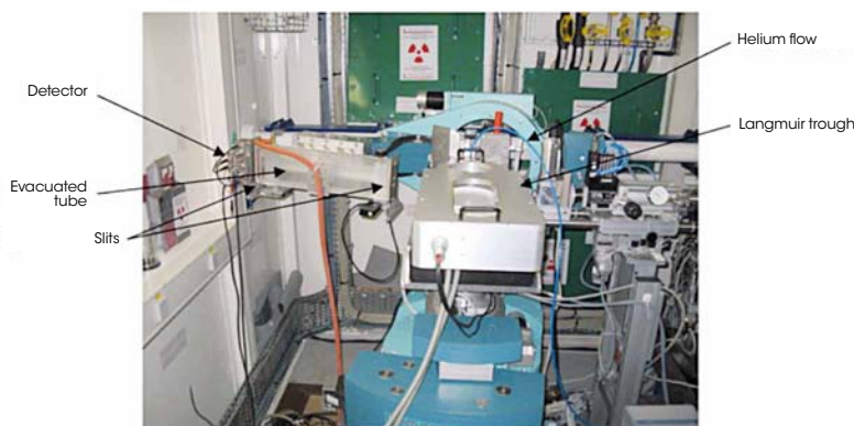
Langmuir trough installed at the ESRF for GISAXS experiment. The same setup will be available on SIRIUS beamline.
