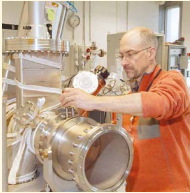
Alain Lestrade doing offset measurements of the DISCO beamline cold finger fiducials
