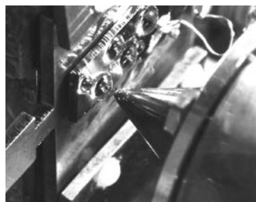
Figure 1: Water droplets on a gold coated silicon surface in the analysis chamber during the acquisition. The soft X-ray beam of TEMPO beamline impinges on the sample from the right. The cone pointing to the droplet is the 300 microns diameter entrance of the electron energy analyzer.
