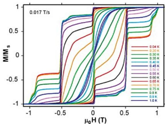
Figure 1. Magnetization curves (i.e. sample magnetization vs. applied magnetic field) of  $Fe_4$  molecule magnet measured on single crystals by microSQUID magnetometry (with a magnetic field sweep rate of 0,017 Tesla/s and at temperatures  $\leq 1$  Kelvin). The presence of hysteresis curves demonstrates the magnetic bistability of  $Fe_4$  at subKelvin temperatures; sharp steps in the hysteresis loops is a proof that the spin dynamic is dominated by quantum effects [ref.1]
