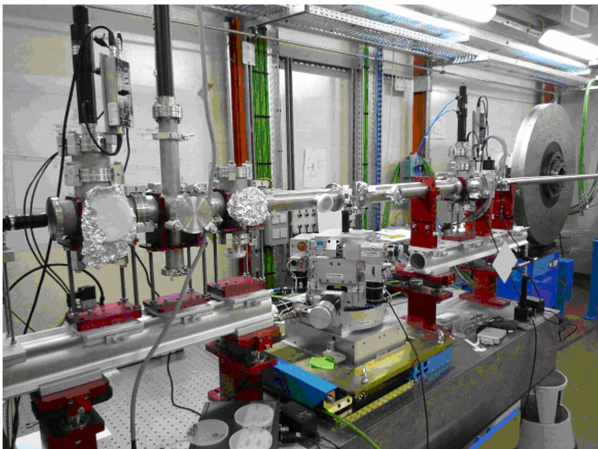
**XAS set up : fluorescence mode (here with a single element SDD)**
